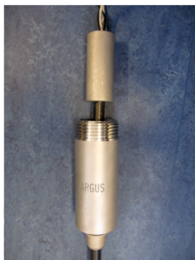
Tension cone inserted into the adapter housing and filled with polyurethane compound
