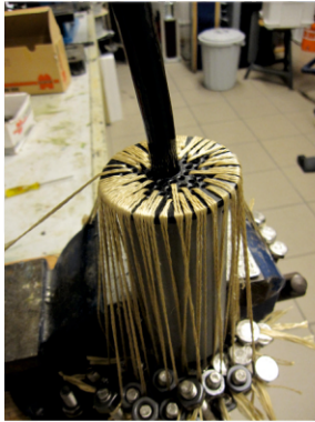
Separating the Kevlar braids before epoxy potting
