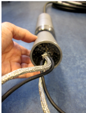
After molding Kevlar ends cut off
