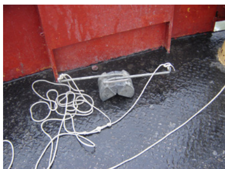
Figure 4.2: Van Veen Grab. Used for taking bed samples.
