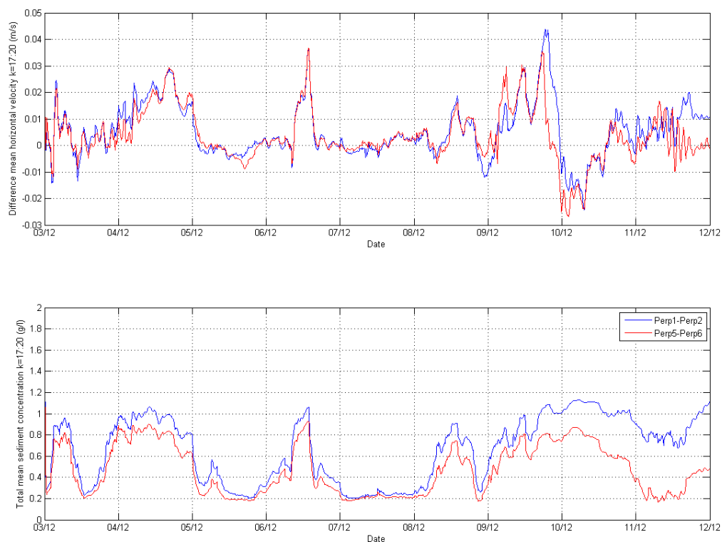
Figure C.13: Density current location (80,78), perpendicular simulation. Same figure as C.12, but in the perpendicular simulation. Results are the same.
