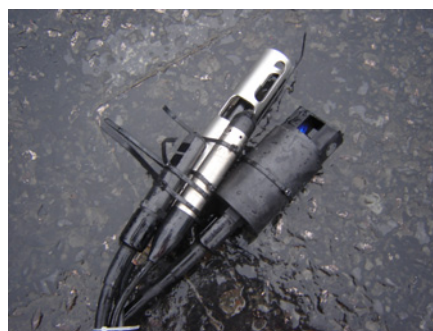
Figure 4.3: CTD, OBS and Chlorophyll sensors. Used for water column measurements.
