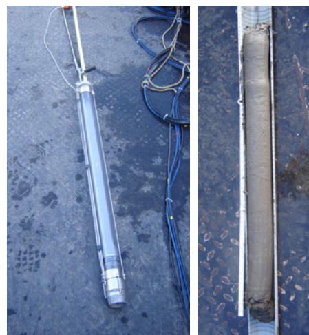
Figure 4.12: Beeker sampler and core in practice.
